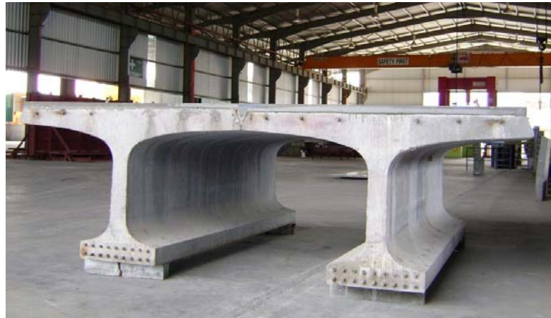
Figure 3 – Photo shows 2 pieces of T875BG joined together.
