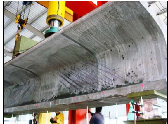
Shear Strength Test Setup For T875BG
