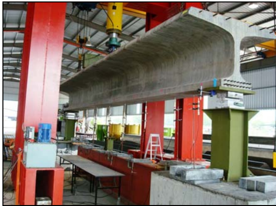
Flexure Strength Test Setup For T875BG
