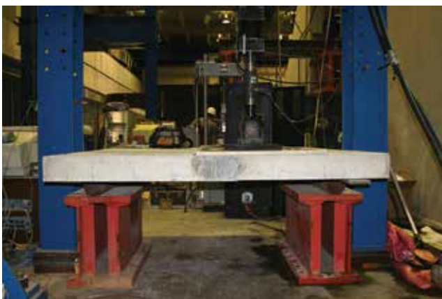
Ultra-high-performance concrete connections are tested in the laboratory at the Turner-Fairbank Highway Research Center in McLean, Va. Courtesy of Ben Graybeal, Federal Highway Administration.
