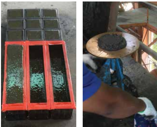
At Dura Technology, grout cubes and beams are cast for compressive and tensile strength testing (left). A worker uses the drop table near the mixer (right). Courtesy of J. P. Binard.
