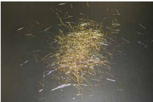
High doses of steel fibers are used in ultra-high-performance concrete to improve ductility and promote a strain-hardening response. Courtesy of Ben Graybeal, Federal Highway Administration.
