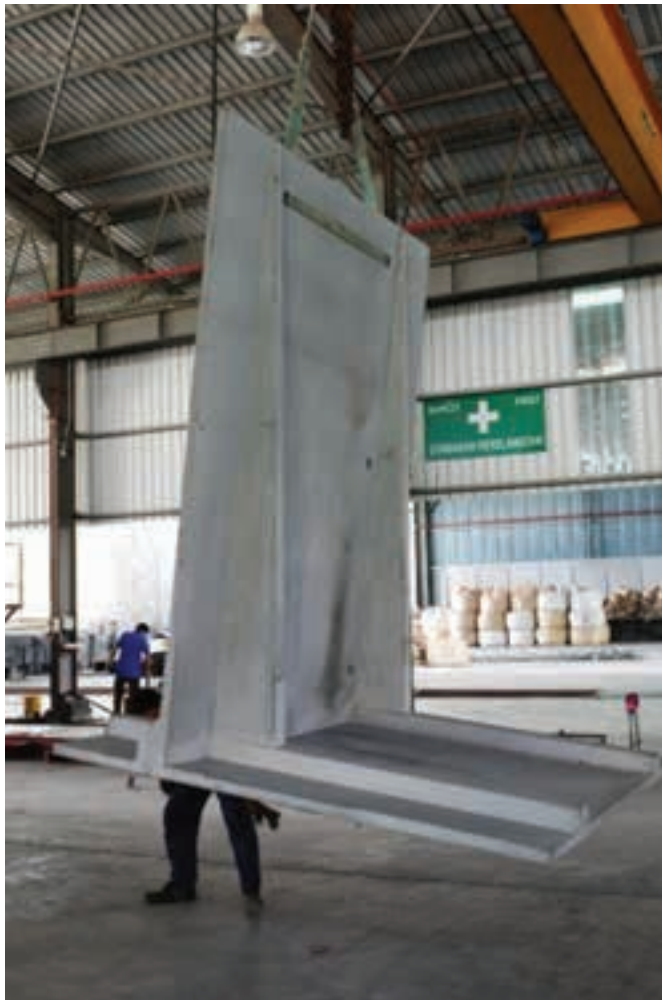
Figure 1: Precast UHPC 2.5 m high retaining wall segment.
