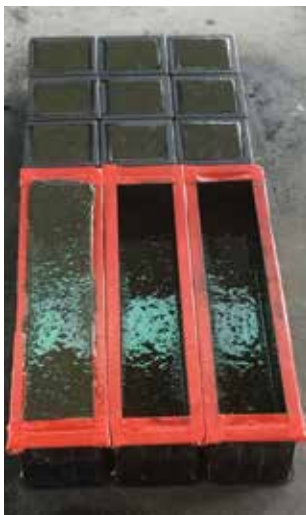
At Dura Technology, grout cubes and beams are cast for compressive and tensile strength testing (left). A worker uses the drop table near the mixer (right). Courtesy of J. P. Binard.
