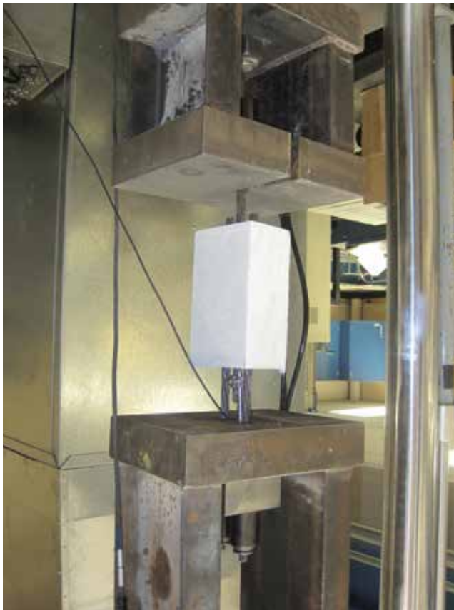
The Federal Highway Administration conducts lap splice tests of untensioned strands at the Turner-Fairbank Highway Research Center as part of the research by Graybeal (2014). Courtesy of Ben Graybeal, Federal Highway Administration.
