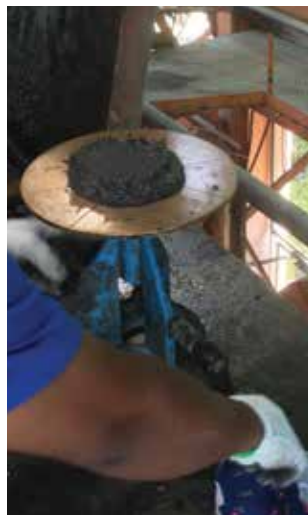
At Dura Technology, grout cubes and beams are cast for compressive and tensile strength testing (left). A worker uses the drop table near the mixer (right). Courtesy of J. P. Binard.
