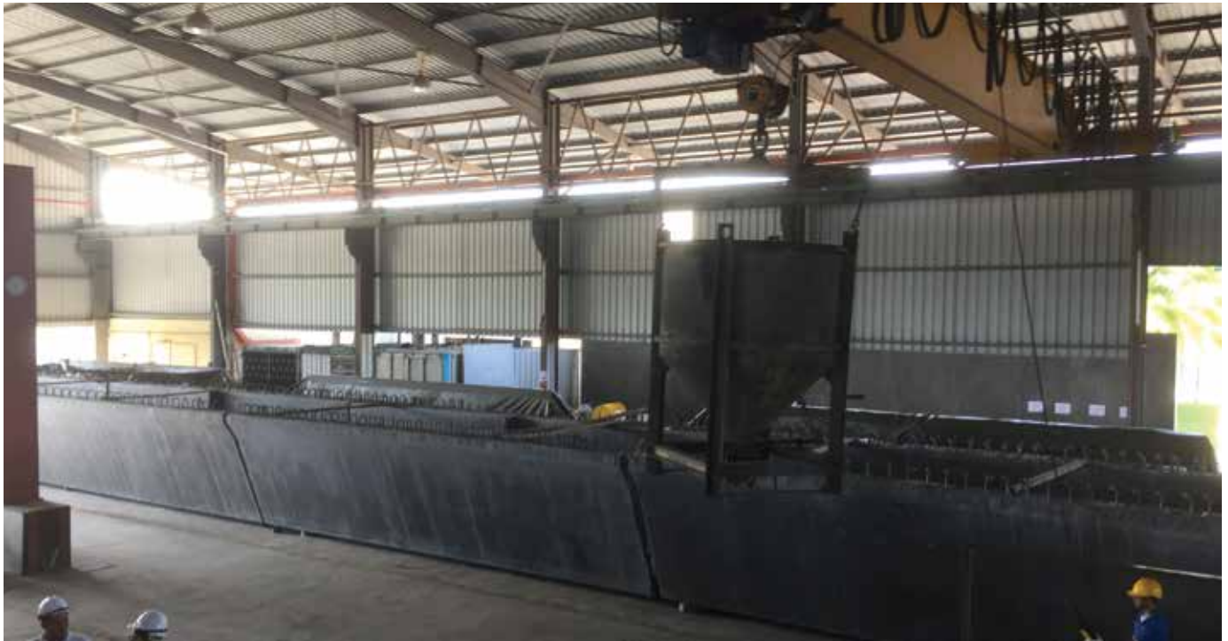
This secondary curing zone at Dura Technology, which is not on the casting beds, is where products are covered and cured in bulk after typical casting and stripping cycles. Courtesy of J. P. Binard.
